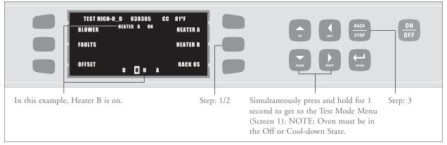
FIGURE 31: Checking Heater B
